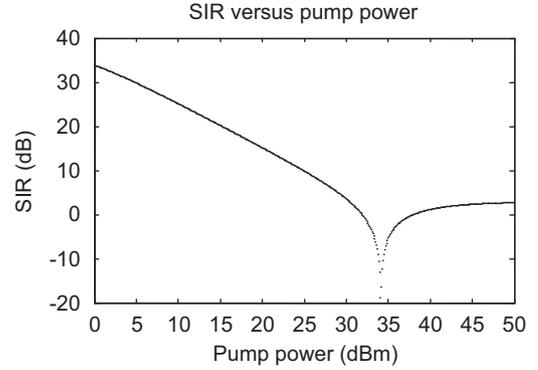
**Fig. 2.** SIR (dB) versus injected pump power (dBm) with injected signal power ( $S_0 = -40 \text{ dBm}$ ) at 400 km,  $\lambda_1 = 1510 \text{ nm}$  and  $\lambda_2 = 1512 \text{ nm}$ .
