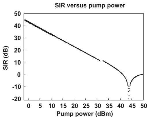
**Fig. 1.** SIR (dB) versus injected pump power (dBm) with injected signal power ( $S_0 = -50 \text{ dBm}$ ) at 400 km,  $\lambda_1 = 1510 \text{ nm}$  and  $\lambda_2 = 1512 \text{ nm}$ .
