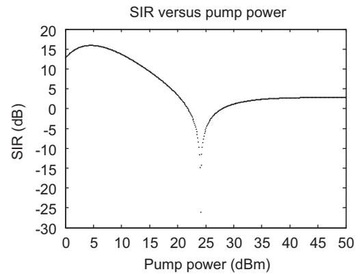
**Fig. 3.** SIR (dB) versus injected pump power (dBm) with injected signal power ( $S_0 = -30 \text{ dBm}$ ) at 400 km,  $\lambda_1 = 1510 \text{ nm}$  and  $\lambda_2 = 1512 \text{ nm}$ .
