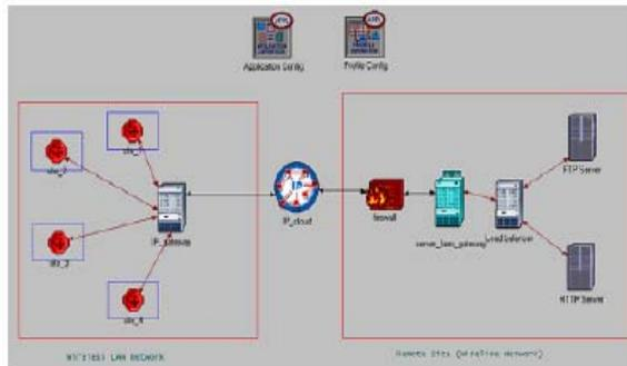
Fig. 2. OPNET Model with load balancer.
