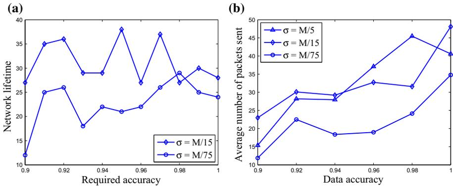
**Fig. 10** Correlation of data with respect to data accuracy for different values of  $\sigma$ . **a** Variation of network lifetime, **b** variation of average number of message transmissions
