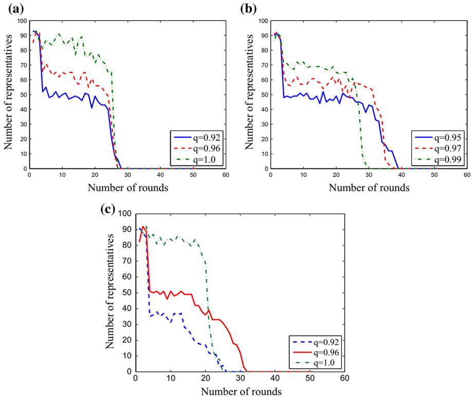
**Fig. 7** Variation of number of Representative with data accuracy at different radio coverage. **a** Radio range  $R = 9$ . **b** Radio range  $R = 12$ . **c** Radio range  $R = 15$
