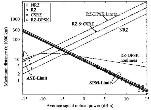
**Fig. 6.** At 10 Gb/s, SPM-limited transmission distance versus launched optical power for various data formats showing SPM limit and ASE limit.
