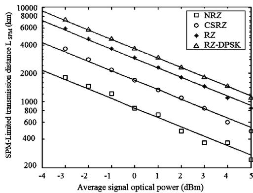
**Fig. 5.** At 40 Gb/s, SPM-limited transmission distance versus launched optical power for various data formats.
