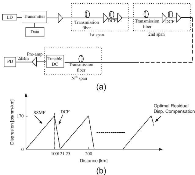
Fig. 1. (a) Schematic of simulation setup. (b) Dispersion map of the simulation setup
