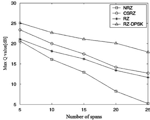
**Fig. 3.** At 40 Gb/s, maximum  $Q$  value versus number of fiber spans for various data formats.
