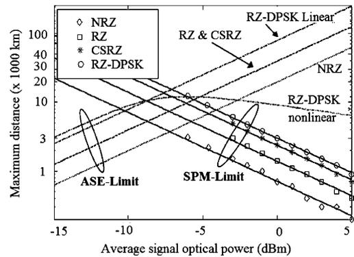
**Fig. 7.** At 40 Gb/s, SPM-limited transmission distance versus launched optical power for various data formats showing SPM limit and ASE limit.
