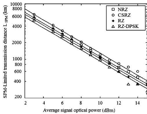
**Fig. 4.** At 10 Gb/s, SPM-limited transmission distance versus launched optical power for various data formats.
