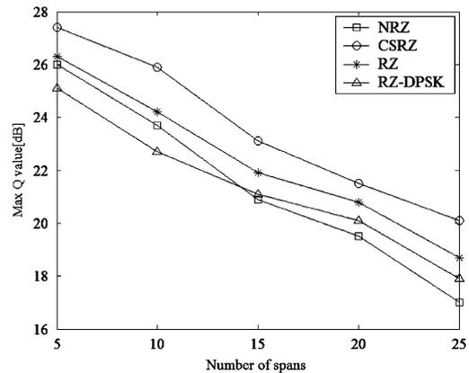
Fig. 2. At 10 Gb/s, maximum  $Q$  value versus number of fiber spans for various data formats.
