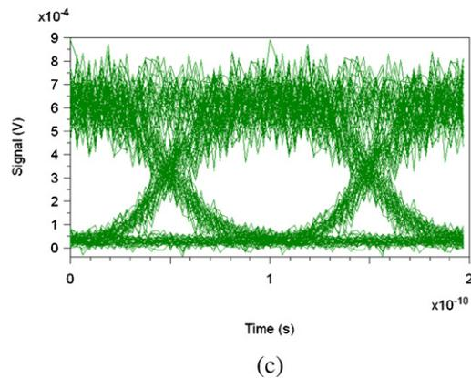
**Fig. 4.** (a) Initial eye opening; (b) frequency chirp signal and (c) eye opening at output.
