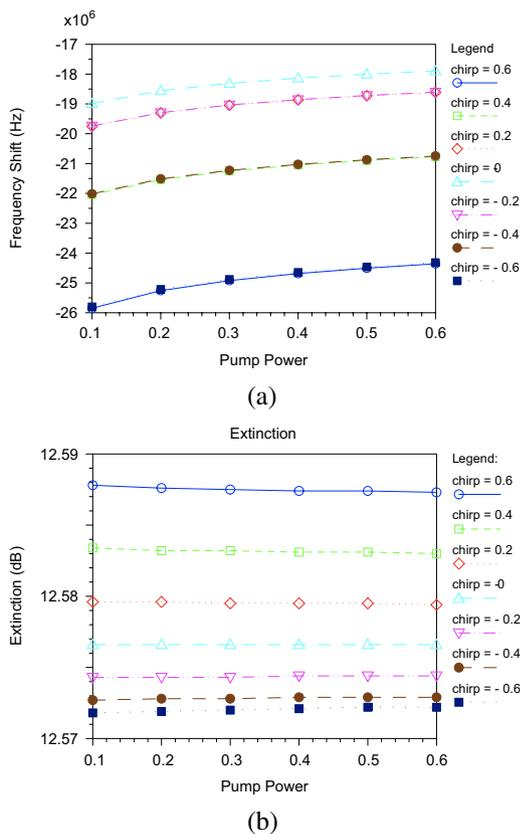
**Fig. 6.** (a) Pump power (dBm) versus frequency shift and (b) pump power (dBm) versus extinction ratio at varied chirp factor.
