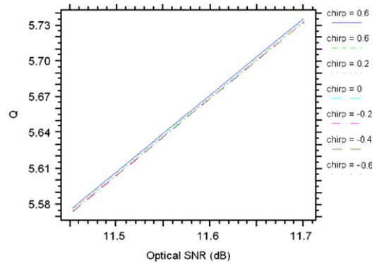
**Fig. 7.** Optical SNR versus  $Q$ -factor at varied chirp factor.
