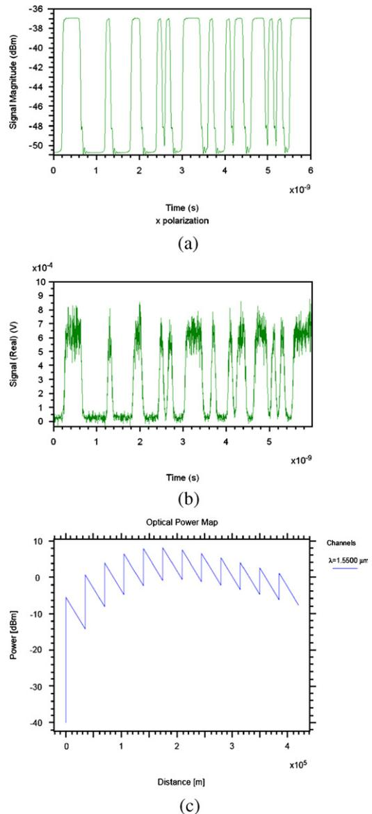
Fig. 3. (a) Input and (b) output at 500 km with ASE and (c) power map.
