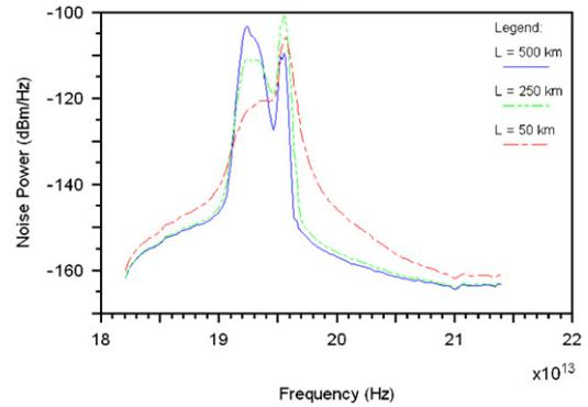
Fig. 2. Illustrates the phenomenon where the ASE output spectral peak gradually shifts to shorter frequencies (longer wavelengths).
