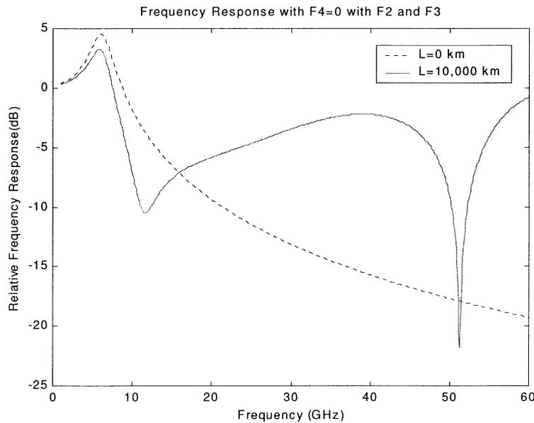
Fig. 4. Small-signal frequency response according to Eq. (35) for  $L = 0$  km and  $L = 10,000$  km with  $S_0 = 0.085$  ps/nm<sup>2</sup>/km,  $d\tau/d\lambda = 5 \times 10^{-3}$  ps/nm/km,  $d^2\tau/d\omega^2 = 0.138$  ps<sup>3</sup>/km, and  $d^3\tau/d\omega^3 = 0.1637$  ps<sup>4</sup>/km. F2 and F3.
