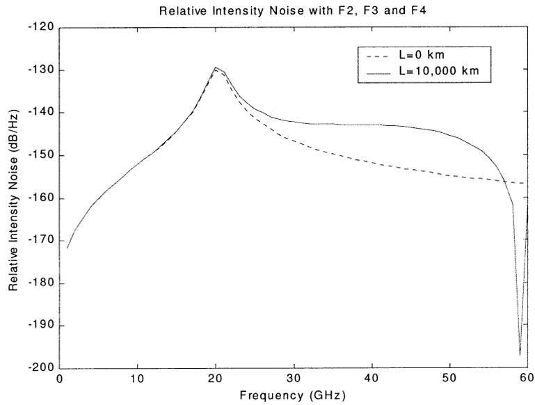
Fig. 13. Small-signal relative intensity noise (RIN) response according to Eq. (46) for  $L = 0$  km and  $L = 10,000$  km with  $S_0 = 0.085$  ps/nm<sup>2</sup>/km,  $d\tau/d\lambda = 5 \times 10^{-3}$  ps/nm/km,  $d^2\tau/d\omega^2 = 0.138$  ps<sup>3</sup>/km, and  $d^3\tau/d\omega^3 = 0.1637$  ps<sup>4</sup>/km. F2, F3, and F4.
