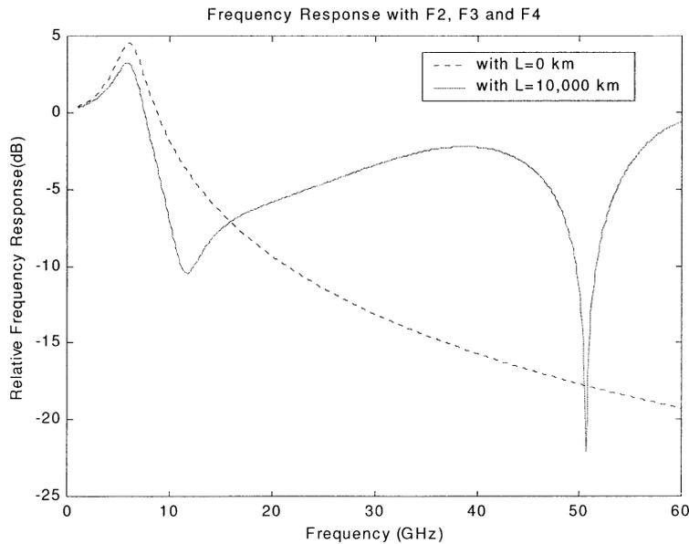
Fig. 6. Small-signal frequency response according to Eq. (35) for  $L = 0$  km and  $L = 10,000$  km with  $S_0 = 0.085$  ps/nm<sup>2</sup>/km,  $d\tau/d\lambda = 5 \times 10^{-3}$  ps/nm/km,  $d^2\tau/d\omega^2 = 0.138$  ps<sup>3</sup>/km, and  $d^3\tau/d\omega^3 = 0.1637$  ps<sup>4</sup>/km. F2, F3, and F4.
