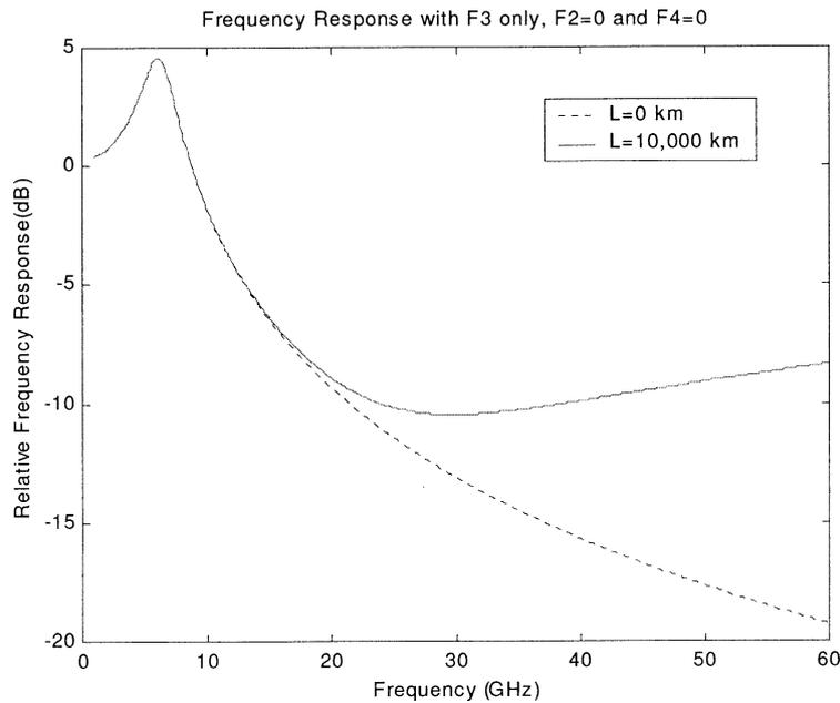
Fig. 2. Small-signal frequency response according to Eq. (35) for  $L = 0$  km and  $L = 10,000$  km with  $S_0 = 0.085$  ps/nm<sup>2</sup>/km,  $d\tau/d\lambda = 5 \times 10^{-3}$  ps/nm/km,  $d^2\tau/d\omega^2 = 0.138$  ps<sup>3</sup>/km, and  $d^3\tau/d\omega^3 = 0.1637$  ps<sup>4</sup>/km. F3 only.
