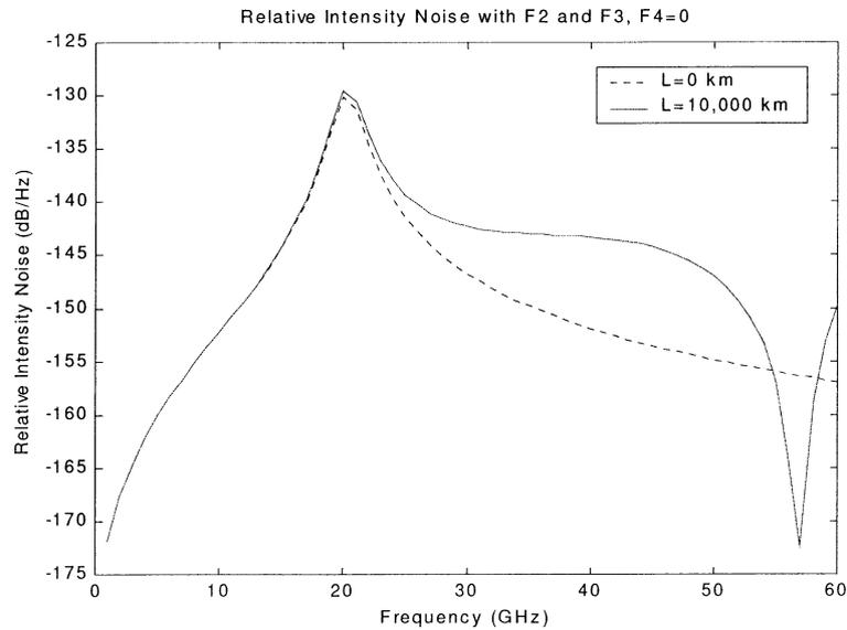
Fig. 11. Small-signal relative intensity noise (RIN) response according to Eq. (46) for  $L = 0$  km and  $L = 10,000$  km with  $S_0 = 0.085$  ps/nm<sup>2</sup>/km,  $d\tau/d\lambda = 5 \times 10^{-3}$  ps/nm/km,  $d^2\tau/d\omega^2 = 0.138$  ps<sup>3</sup>/km, and  $d^3\tau/d\omega^3 = 0.1637$  ps<sup>4</sup>/km. F2 and F3.
