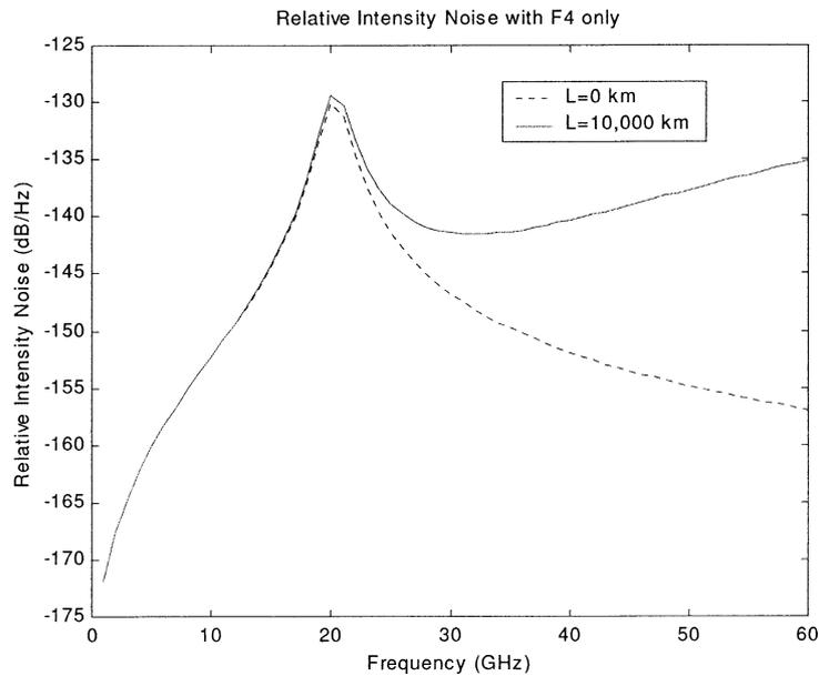
Fig. 10. Small-signal relative intensity noise (RIN) response according to Eq. (46) for  $L = 0$  km and  $L = 10,000$  km with  $S_0 = 0.085$  ps/nm<sup>2</sup>/km,  $d\tau/d\lambda = 5 \times 10^{-3}$  ps/nm/km,  $d^2\tau/d\omega^2 = 0.138$  ps<sup>3</sup>/km, and  $d^3\tau/d\omega^3 = 0.1637$  ps<sup>4</sup>/km. F4 only.
