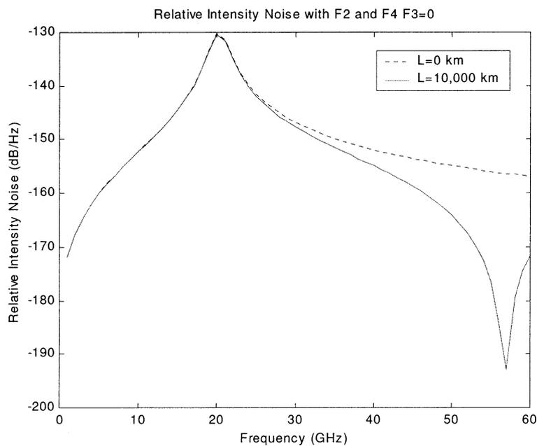
Fig. 12. Small-signal relative intensity noise (RIN) response according to Eq. (46) for  $L = 0$  km and  $L = 10,000$  km with  $S_0 = 0.085$  ps/nm<sup>2</sup>/km,  $d\tau/d\lambda = 5 \times 10^{-3}$  ps/nm/km,  $d^2\tau/d\omega^2 = 0.138$  ps<sup>3</sup>/km, and  $d^3\tau/d\omega^3 = 0.1637$  ps<sup>4</sup>/km. F2 and F4.
