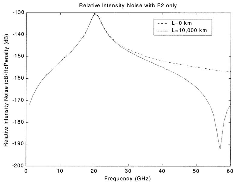
Fig. 8. Small-signal relative intensity noise (RIN) response according to Eq. (46) for  $L = 0$  km and  $L = 10,000$  km with  $S_0 = 0.085$  ps/nm<sup>2</sup>/km,  $d\tau/d\lambda = 5 \times 10^{-3}$  ps/nm/km,  $d^2\tau/d\omega^2 = 0.138$  ps<sup>3</sup>/km, and  $d^3\tau/d\omega^3 = 0.1637$  ps<sup>4</sup>/km. F2 only.
