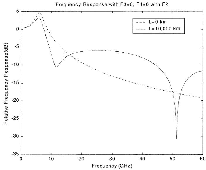
Fig. 1. Small-signal frequency response according to Eq. (35) for  $L = 0$  km and  $L = 10,000$  km with  $S_0 = 0.085$  ps/nm<sup>2</sup>/km,  $d\tau/d\lambda = 5 \times 10^{-3}$  ps/nm/km,  $d^2\tau/d\omega^2 = 0.138$  ps<sup>3</sup>/km, and  $d^3\tau/d\omega^3 = 0.1637$  ps<sup>4</sup>/km. F2 only.
