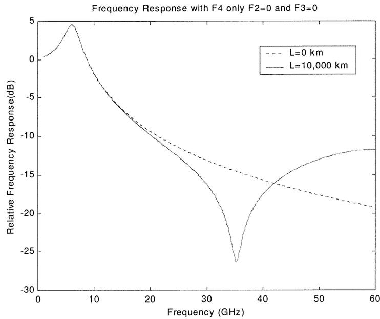
Fig. 3. Small-signal frequency response according to Eq. (35) for  $L = 0$  km and  $L = 10,000$  km with  $S_0 = 0.085$  ps/nm<sup>2</sup>/km,  $d\tau/d\lambda = 5 \times 10^{-3}$  ps/nm/km,  $d^2\tau/d\omega^2 = 0.138$  ps<sup>3</sup>/km, and  $d^3\tau/d\omega^3 = 0.1637$  ps<sup>4</sup>/km. F4 only.
