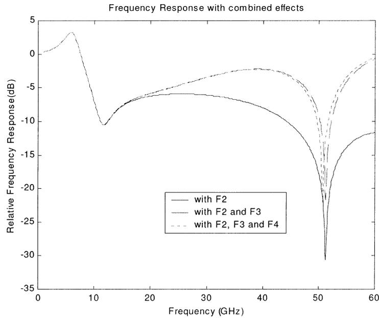
Fig. 7. Small-signal frequency response according to Eq. (35) for  $L = 0$  km and  $L = 10,000$  km with  $S_0 = 0.085$  ps/nm<sup>2</sup>/km,  $d\tau/d\lambda = 5 \times 10^{-3}$  ps/nm/km,  $d^2\tau/d\omega^2 = 0.138$  ps<sup>3</sup>/km, and  $d^3\tau/d\omega^3 = 0.1637$  ps<sup>4</sup>/km. Combined effects.
