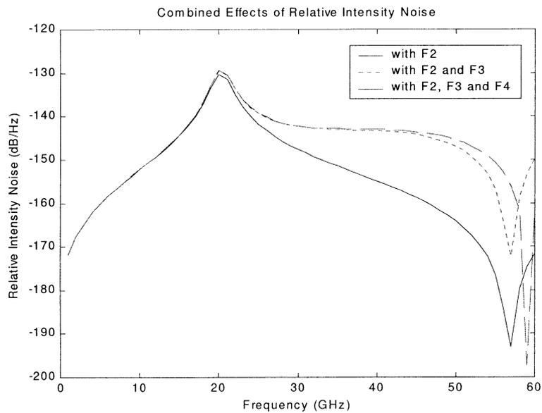
Fig. 14. Small-signal relative intensity noise (RIN) response according to Eq. (46) for  $L = 0$  km and  $L = 10,000$  km with  $S_0 = 0.085$  ps/nm<sup>2</sup>/km,  $d\tau/d\lambda = 5 \times 10^{-3}$  ps/nm/km,  $d^2\tau/d\omega^2 = 0.138$  ps<sup>3</sup>/km, and  $d^3\tau/d\omega^3 = 0.1637$  ps<sup>4</sup>/km. Combined effects.
