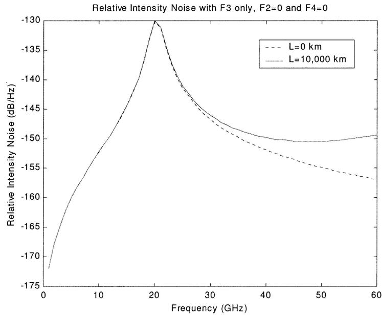
Fig. 9. Small-signal relative intensity noise (RIN) response according to Eq. (46) for  $L = 0$  km and  $L = 10,000$  km with  $S_0 = 0.085$  ps/nm<sup>2</sup>/km,  $d\tau/d\lambda = 5 \times 10^{-3}$  ps/nm/km,  $d^2\tau/d\omega^2 = 0.138$  ps<sup>3</sup>/km, and  $d^3\tau/d\omega^3 = 0.1637$  ps<sup>4</sup>/km. F3 only.
