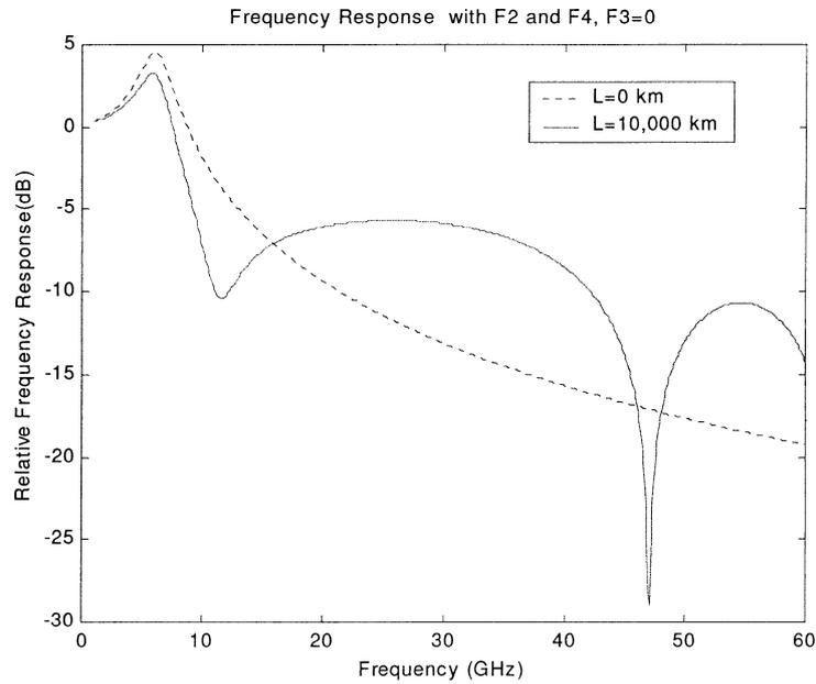
Fig. 5. Small-signal frequency response according to Eq. (35) for  $L = 0$  km and  $L = 10,000$  km with  $S_0 = 0.085$  ps/nm<sup>2</sup>/km,  $d\tau/d\lambda = 5 \times 10^{-3}$  ps/nm/km,  $d^2\tau/d\omega^2 = 0.138$  ps<sup>3</sup>/km, and  $d^3\tau/d\omega^3 = 0.1637$  ps<sup>4</sup>/km. F2 and F4.
